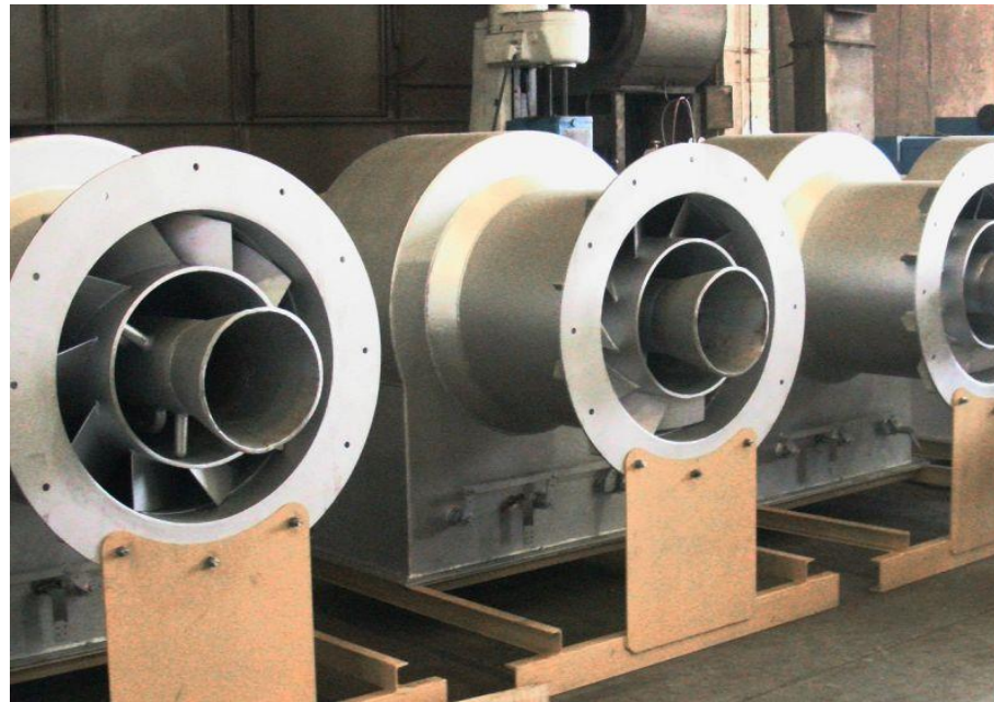
22 MW th burners for biomass combustion
